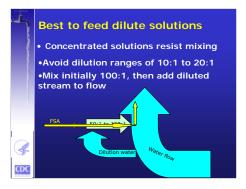
Concentrated solutions do resist mixing. If you have long pipe runs with several twists and turns, the solution will eventually mix, but if you want to ensure a rapid and consistent mixing, then use a dilution flow to dilute the concentrated FSA before adding to the main flow stream. Mix in the range of 100 to 1, avoiding the danger zone of 10:1 to 20:1 when scaling can occur.
