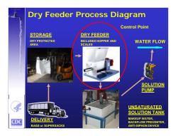
When sodium fluorosilicate is the additive of choice, the process can be quite simple. The additive, in bags or supersacks, is delivered to the facility. The material is dispensed by the dry feeder at a regulated rate, and is mixed with water in a solution tank to an unsaturated solution. Then it is fed to the plant flow. The control point is the dry feeder.
