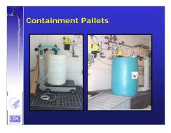
All tanks should have containment in the event of a spill. Commercially available containment pallets can provide secure protection for various sizes of tanks and totes. Be sure to have a containment pallet sufficient to hold the entire contents of the drum or container in the event of a spill.
