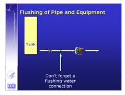
When installing the equipment and piping, remember that it will be necessary to maintain or repair the equipment, and the solutions are potentially hazardous to personnel. Remember to install a flushing water connection so that pipes and equipment can be cleaned before being disassembled.
