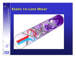
A static mixer is a screw-like vane pipe insert to promote mixing of the solution with the water flow. This is particularly important if the first customer is only a short distance downstream from the facility.
