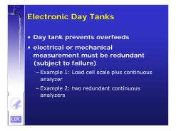
Can you use an electronic day tank to avoid the cost of a separate tank and the associated equipment. Electronic devices are subject to failure, so you would need a redundant measurement to verify that an excessive feed is not occurring. This could be a load cell set for pre-determined maximum weight loss in a certain time interval plus a continuous analyzer, or two redundant continuous analyzers.
