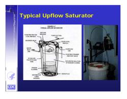
By the 1980s, the downflow saturator had been replaced by the upflow saturator mainly because of operation and maintenance problems with the downflow saturator. One big advantage is that the sand and gravel were eliminated. But the inlet waterline is plumbed directly to the distribution piping at the bottom of the tank and, with no air gap possible, a vacuum breaker and backflow preventer are needed. This is one type of upflow saturator, but there are different varieties on the market.
