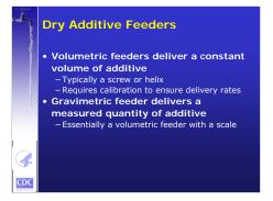
Volumetric feeders deliver a constant volume, but they require periodic recalibration to ensure a consistent delivery. Historically, volumetric feeders are the most common device for chemical metering in water plants due to their lower cost.
