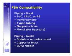
PVC, CPVC or Polyethylene piping is commonly used for FSA solutions, but polypropylene can also be used. PVC has been more commonly used, but its disadvantages are that it is a rigid connection with many joints for potential leaking where polyethylene is a flexible piping. Tygon tubing and neoprene rubber hoses can also be used, but typically used for hose or peristaltic pumps. Monel, a nickel-rich steel alloy, is FSA resistant and is suitable as an injector.
