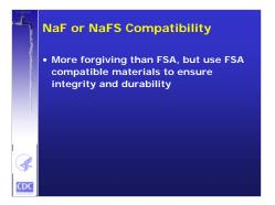
Sodium fluoride and sodium fluorosilicate solutions are more forgiving than FSA, due to their moderate pH and the absence of hydrogen fluoride, but the best practice is to stick with the same materials as would be suitable for FSA. By doing this, if there is ever the need to change additives, the system will already be compatible.
