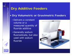
Dry feeders deliver a constant volume of fluoride additive and generally are used with sodium fluorosilicate; they can also be used with sodium fluoride.
