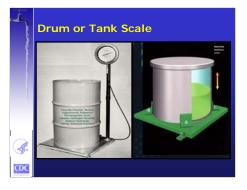
Scales for drums and tanks are an excellent means of accurately documenting the use of fluoride solution. An advantage of using scales is that there is nothing extending into the atmosphere of the tank so hydrogen fluoride corrosion is avoided. If your installation does not have a scale, consider adding one for improved management and verification of precise fluoride feed. Scales can be obtained for any size, including for an entire tank. Normally, only a day tank needs to be weighed.
