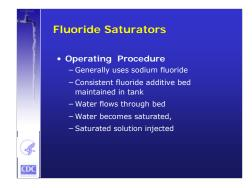
A fluoride saturator, either the downflow or the upflow type, maintains a bed, or layer, of sodium fluoride in a tank. Water flows through the bed and dissolves the sodium fluoride.
