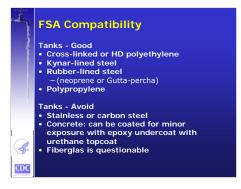
Verify with manufacturers on the compatibility of the materials, but there are some general considerations on acceptable materials of construction. For tanks, cross-linked polyethylene tanks are the best choice for FSA, but polypropylene, rubber-lined steel, or Kynar-lined steel tanks are acceptable. Rubber-lined tanks require inspection and repair of the rubber lining periodically.
