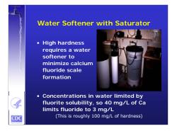
In areas with high hardness, a water softener is often needed on the make-up water feed to minimize the potential for calcium fluoride scale formation. To avoid scale formation in hard water, either a water softener is needed, or FSA would be the system to minimize scale formation. 10-State standards specifies water softening if hardness exceeds 75 mg/L as calcium carbonate.
