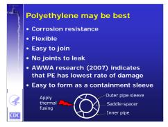
I personally believe polyethylene pipe is the best for fluoridation. It has excellent corrosion resistance, it is flexible, easy to join with a small heating element, no joints to leak which is common with PVC, and AWWA research suggests it has the lowest rate of damage for pipe materials. Also, it is easy to form with a containment sleeve.
