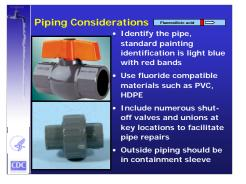
Use fluoride-compatible materials such as polyvinyl chloride (PVC), chlorinated PVC (CPVC), and HDPE in pipe manifolds. Be sure to include numerous shut-off valves and unions at key locations to facilitate pipe repairs. Use a color-coding system to clearly mark that the supply is a fluoride solution. A recommended painting scheme is light blue with red bands, with an arrow indicating the direction of flow and the word "Fluoride" on the pipe.
