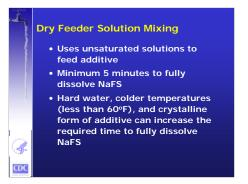
Unlike sodium fluoride, which has a constant solubility, sodium fluorosilicate has a solubility that varies with temperature, from 0.44 g per 100 mL (which is 1/10th that of sodium fluoride) at 32°F to 2.45 g per 100 mL at 212°F. When the water temperature is 77°F, the solubility is approximately 0.762 g per 100 mL, or 1/5th the saturated solution strength of sodium fluoride at the same temperature. Consequently, it requires a lot more water to form a solution.
