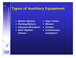
A complete system needs vacuum breakers, anti-siphon valves, and day tanks; it may also include water meters, pacing meters, mixers, scales, and continuous analyzers. As with any process, the more ability the operator has to operate and manage the system, the better will be the results.
