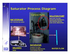
When a saturator is used, the process can be quite simple. The storage area should be convenient to the saturator for ease in filling, and the sodium fluoride is added to the saturator to maintain a uniform bed depth. Makeup water refills the saturator to create a saturated solution. The control point for a saturator is the feed pump which controls the addition of fluoride to the water flow.
