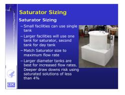
If operated properly, the solution is completely saturated by the time it passes all the way through the bed. For very small communities, the upper portion of the tank can serve as a day tank and the lower portion of the tank as the saturator. Every day, the operator verifies that there is sufficient additive in the bed and then turns on the water to fill the upper portion to the fill line. This displaces the saturated solution in the bed into the day-tank upper portion of the tank.
