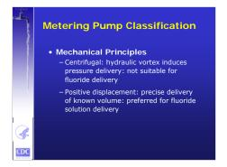
Pumps used to deliver fluoride products to drinking water must be accurate and consistent in their delivery rate. We want to maximize benefits and minimize the risk of fluorosis.
