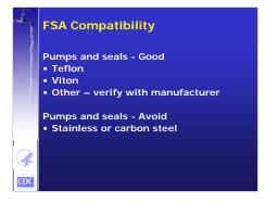
Pump materials can include many materials, considerably beyond what is shown here. In general, Teflon and Viton are both good materials, and other surface treatment may also be suitable. Check with your pump supplier and ensure that the materials are fluoride resistant. Teflon is a polyethylene with fluorine just like PVC is polyethylene with chlorine.
