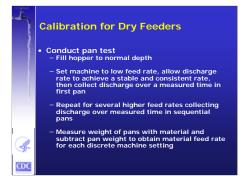
Calibration of dry feeders involves use of a pan test. Here is how a pan test is conducted.
