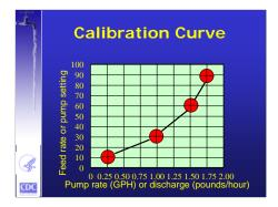
Once you have collected the discharge rate from the pump or the feeder, you can plot the results on a chart. Draw a line between the dots, and you have the result. This chart is prepared plotting the feed rate settings, normally 0%–100%, against either the pumping rate in gallons per minute or the discharge rate in pounds per hour.
