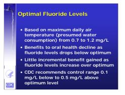
We are adding these compounds to the water so that we can adjust the fluoride concentration to the optimal level for preventing tooth decay. The optimal fluoride level for a location is based on the average maximum daily air temperature, and we use data from a 5-year period. This average is for the entire year; we do not recommend changing the optimal level to account for seasonal temperature variations.
