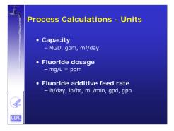
To get the right dosage of fluoride additive, it is necessary to know how much to add. This requires some math, but the calculations are the same type as those required for other chemical additives at a treatment facility. So let's review the simple math calculations that are needed for any process control in a water facility. As is the case with other calculations, it is normally necessary to express the calculations in units of measurement.
