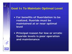
For the full benefits of fluoridation to be realized, fluoride must be maintained at or near the optimal level. For [Georgia], the optimal level is [0.80] mg/L. The principal reason for low or erratic fluoride levels is poor operation and maintenance.
