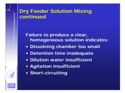
It is important that the dry additive be fully dissolved and not fed to the water flow as a partially dissolved slurry. If the solution is not a clear, homogeneous solution, then one of several things likely needs to be changed.
